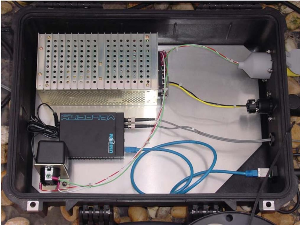
Figure 4. Internal configuration of re-designed conversion box.
